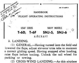
(2) CROSS-WIND LANDING.—As this airplane has a landing gear of normal tread, cross-wind landings may be negotiated safely. Keep one wing down, into the wind, to counteract drift.
