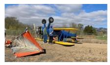
General Aviation has 5 ground loops a week on average over the last 20 years (Aviation Safety Magazine) a large portion of these occur using the wheel landing crosswind technique. How
