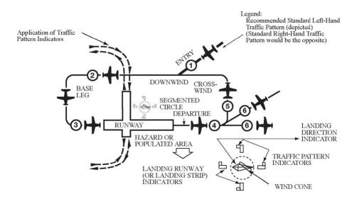
The notes accompanying this depiction all plainly say the primary entry to the non-towered traffic pattern is the 45 degree to downwind at mid-field and at pattern altitude. Additionally, the FAA guidance is to enter "well clear" of traffic already established in the traffic pattern. In my first article about non-towered operations, I referenced CFR 14-Part 91.126/127 and that
